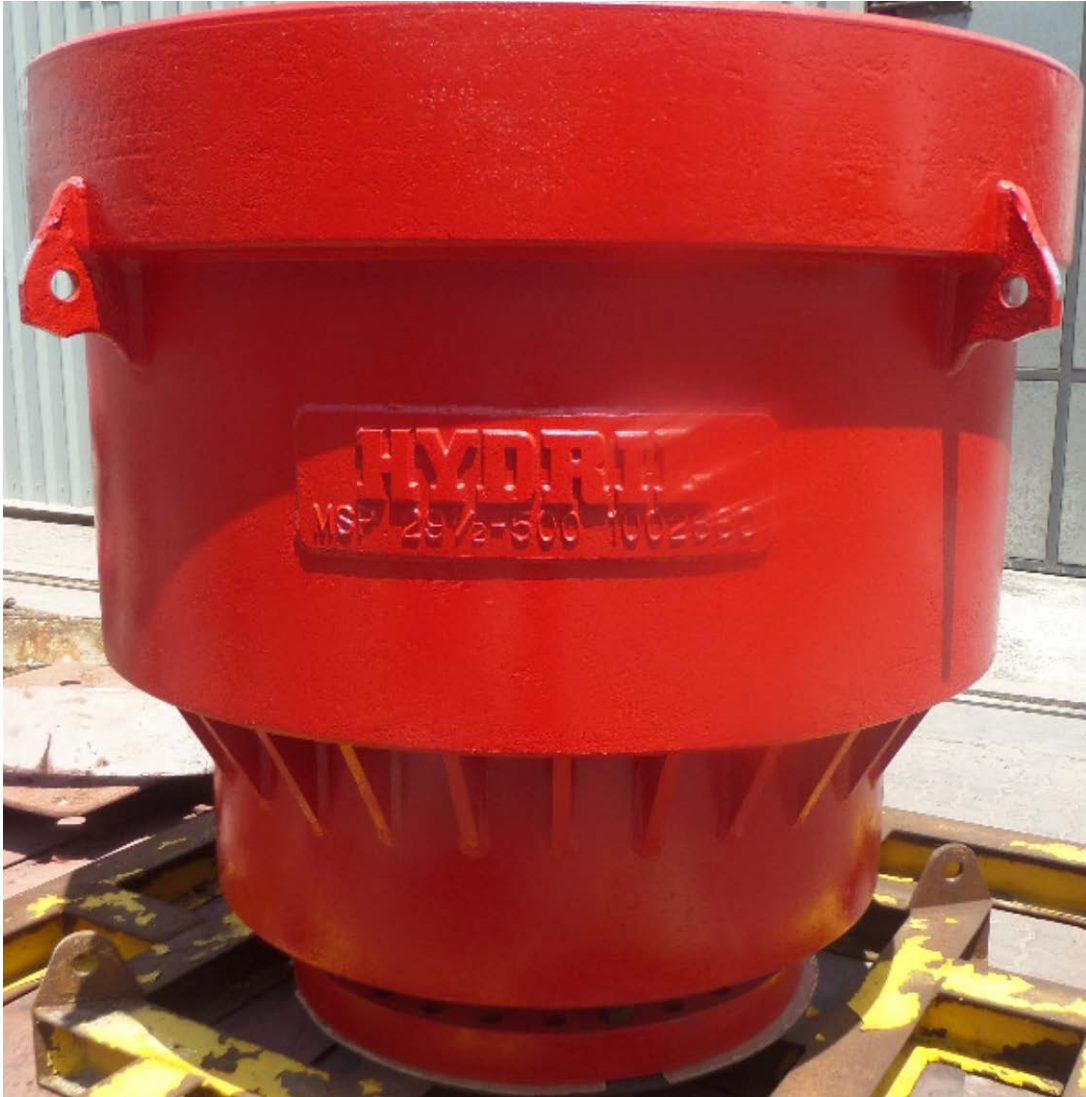
HYDRIL 29-1/2" 500 "MSP" DIVERTER S/N-46528 , P/N- 1002660 QTY: 01 Assy.
