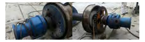
e. Cathead shaft already dismounted to remove the worn bearings
