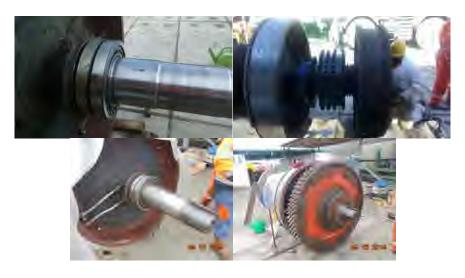
h. High speed clutch removed and found with some broken pads. Replace all the pad
