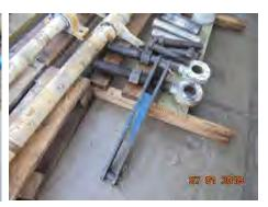
q. Funded brake lever supports with bushings worn by foreign materials. Advise to replace
